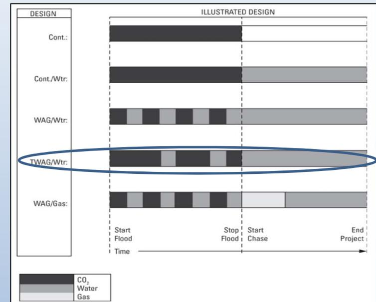
CO<sub>2</sub> Flood and Injection Designs Schematic (Jarrell et al., 2002)
