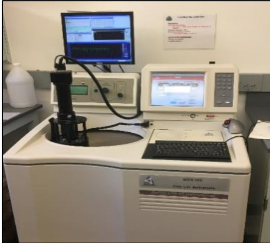
Core Laboratories ACES-200 ultra-high-speed centrifuge (Uzun 2018)
