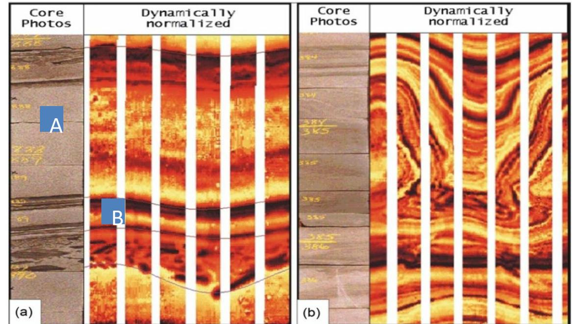
**FIGURE 4.74** (a) Borehole-image log illustrating an erosional surface lined with shale clasts, as calibrated to a core in the same interval. (b) Borehole-image log illustrating a contorted (slumped) bedset; the slumped beds are more easily recognized on the borehole-image log than in the core! This example is from the Cretaceous Lewis Shale, Wyoming. *Images and photographs provided by S. Goolsby.*
