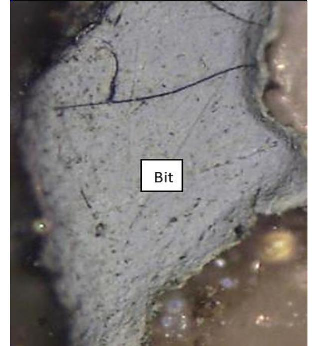
The above values were measured on bitumen. The VRo-eq is estimated to be 1.17% using the Jacob formula ( $R_{vit} = R_{bit} \times 0.618 + 0.4$ ).
