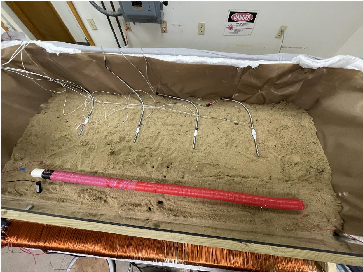
Figure B.1 This figure shows the sandbox experimental setup. Temperature probes are evenly spaced at the top of the box. The solenoid is shown near the bottom of the box. The DMS fiber is buried shallow between the solenoid and temperature probes
