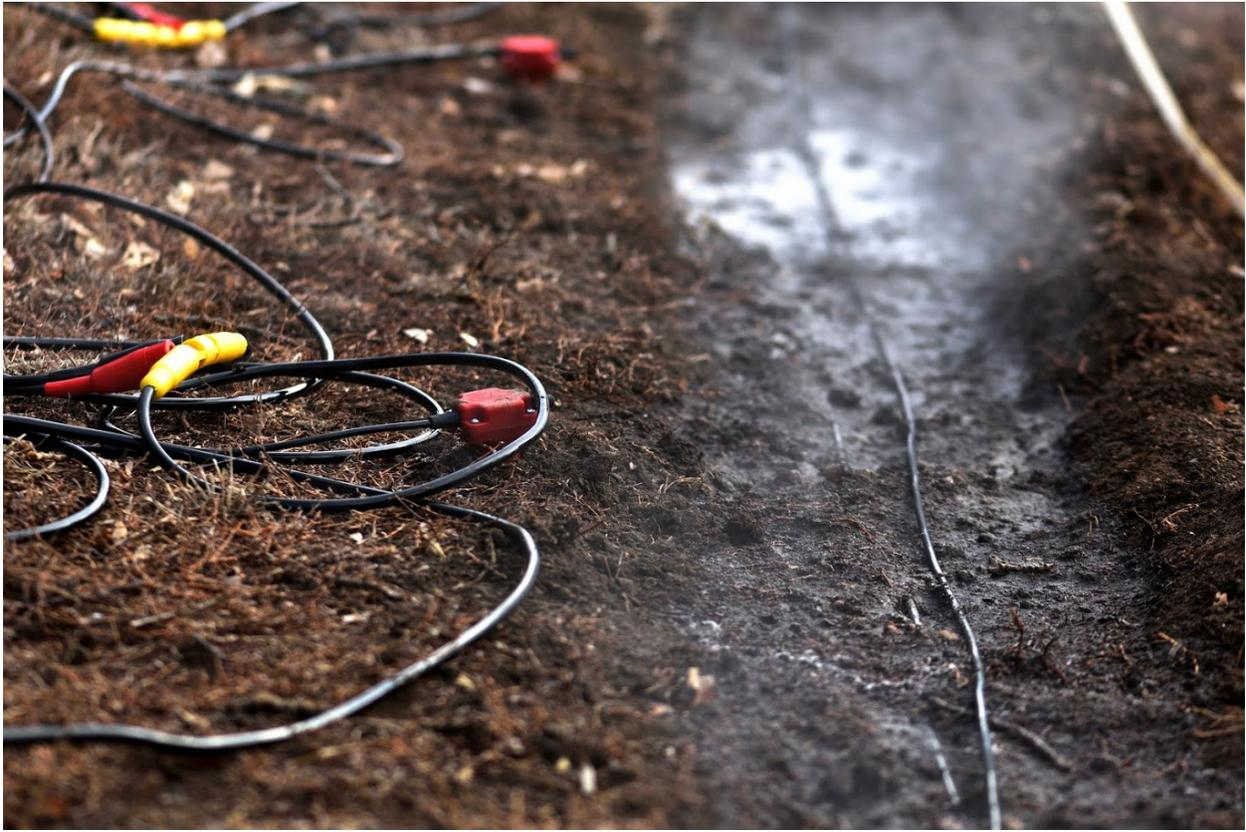
**Figure 1.** Fiber on Section B with the deployed geophones to the left. The steam is from hot water poured on the ground to eventually freeze the fiber to improve ground-fiber coupling. (Photo credit: Iga Pawelec)
