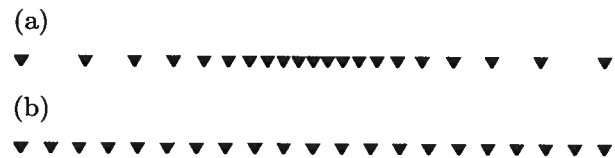
Figure 3. 2D surface array for optimized design (a) and conventional design (b). The optimized array is designed for a hypocentral depth of 1800 m, maximum offset of 6000 m and a constant velocity gradient of \approx 1.3 \text{ s}^{-1} .
