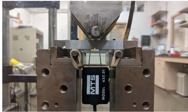
Figure 7.8 Three point bending fracture test setup.
