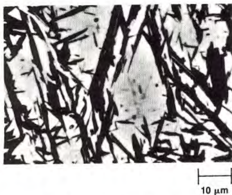
Fig 17 High retained austenite content in corner of SAE 4121 steel (formerly EX24) specimen carburized at 1050 °C (1920 °F). Source: Ref 44
