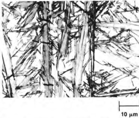
Fig 15 Microcracks in martensite plates of an Fe-1.86C alloy. Light micrograph. Source: Ref 42
