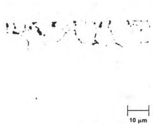
Fig 24 Internal oxidation (dark features) at surface of gas-carburized steel containing 1.06% Mn, 0.21% Si, 0.52% Cr, 0.50% Ni, and 0.17% Mo. Light micrograph. Source: Ref 20
