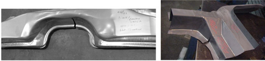
Fig. 4.40 Cracks observed in formed parts initiated at sheared edges [103]
