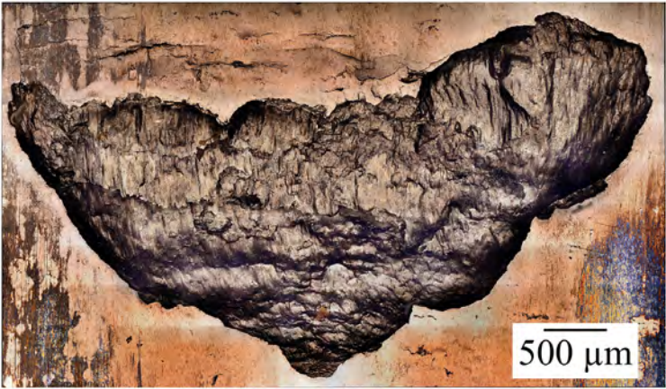
FIG. 17 Light optical microscope image of the pit that developed along the wear track of the tested 4320 steel bar. The machine used to capture the image was a Keyence VHX-5000. The direction of load movement is up.
