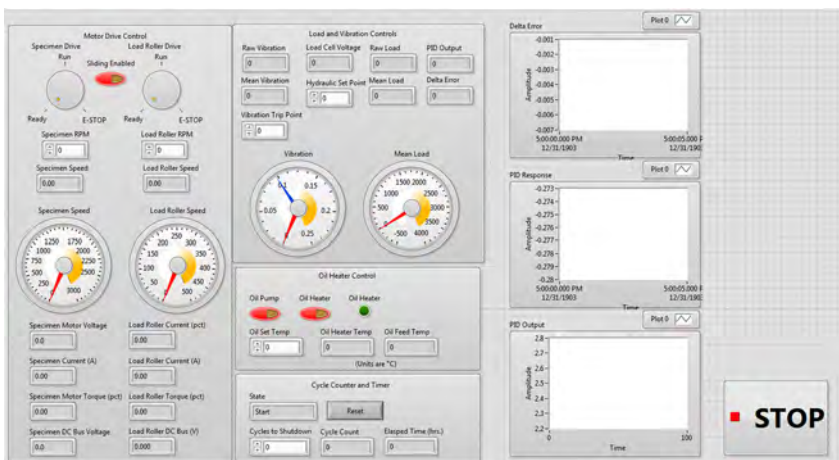
FIG. 6 Front panel of the LabVIEW program used to control the machine.
