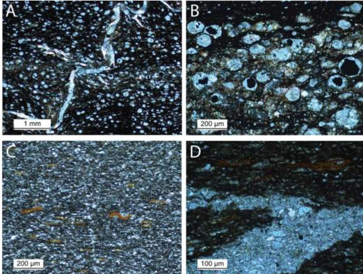
Thin section photomicrographs from the Clarion Mertes core with images from high-silica samples on top and low-silica samples on the bottom
