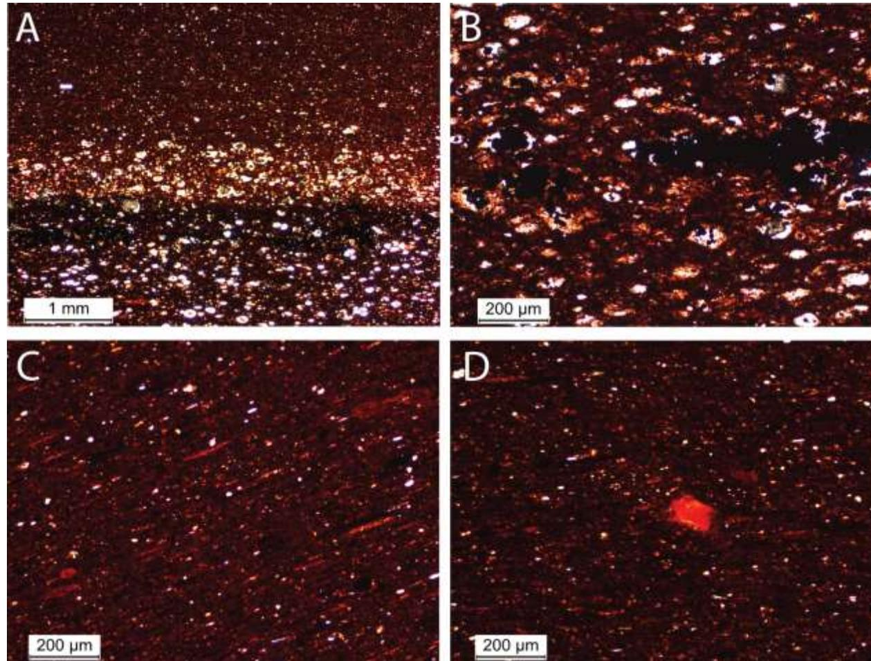
Thin section photomicrographs from the Koch core with images from high-silica samples on top and low-silica samples on the bottom
