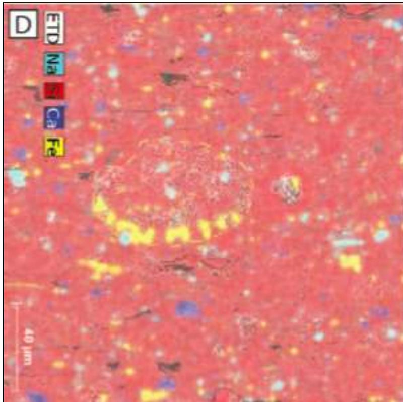
X-ray elemental map of a dissolved radiolarian test (dashed line) being replaced by pyrite in the Mowry shale (*Milliken and Olsen, 2017*)
