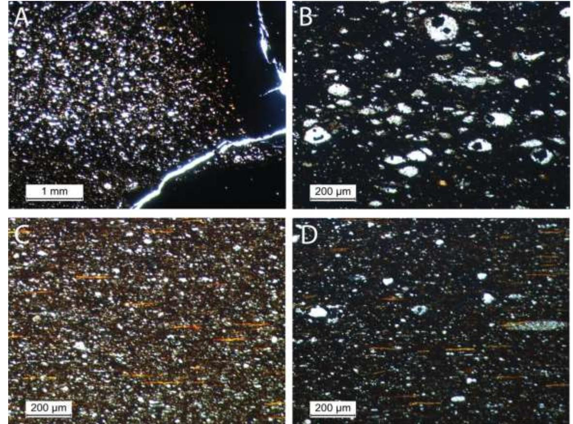
Thin section photomicrographs from the Harvey Grey core with images from high-silica samples on top and low-silica samples on the bottom
