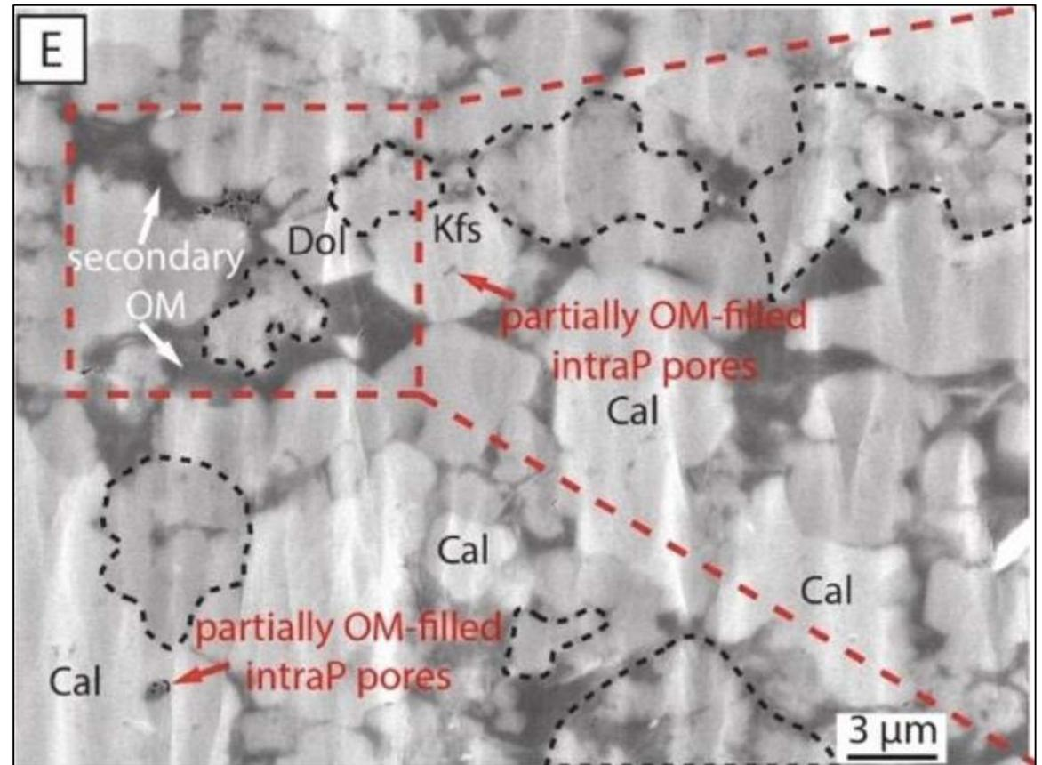
SEM Photomicrograph of authigenic microquartz (dashed lines), K-feldspar, calcite, and organic matter (*Xu, 2019*)
