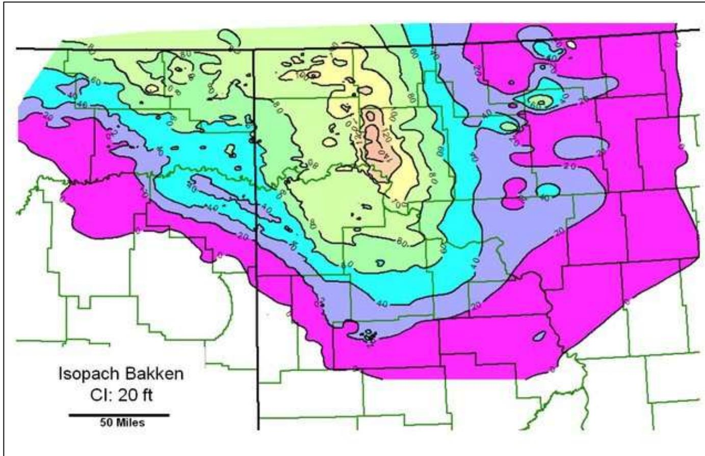
Isopach Map of the Bakken Formation. Thickness ranges from wedge-edge to over 140 feet. From Sonnenberg et al., 2011
