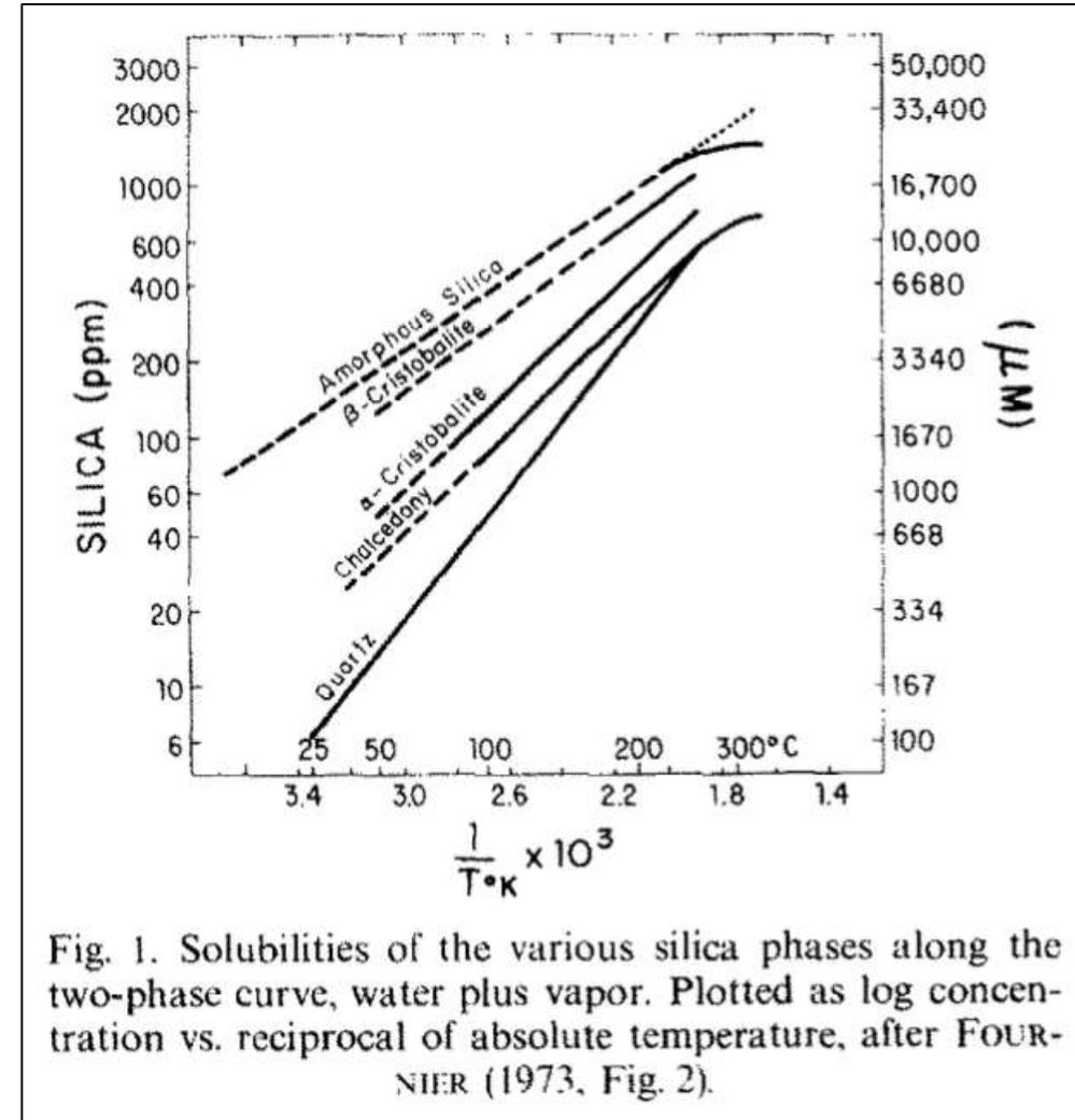
Fig. 1. Solubilities of the various silica phases along the two-phase curve, water plus vapor. Plotted as log concentration vs. reciprocal of absolute temperature, after FOURNIER (1973, Fig. 2).
