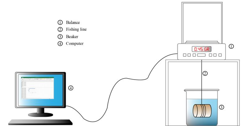
**Saturation Measurement Apparatus**
