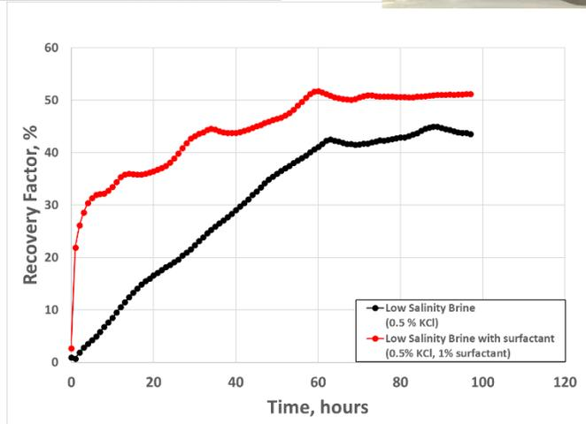
Low salinity brine with non-ionic surfactant increases hydrocarbon recovery with additional 6%
