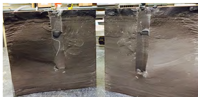
Fig. 11—Fracture plane after breakdown fracturing of the untreated-shale specimen (Specimen No. S4).
