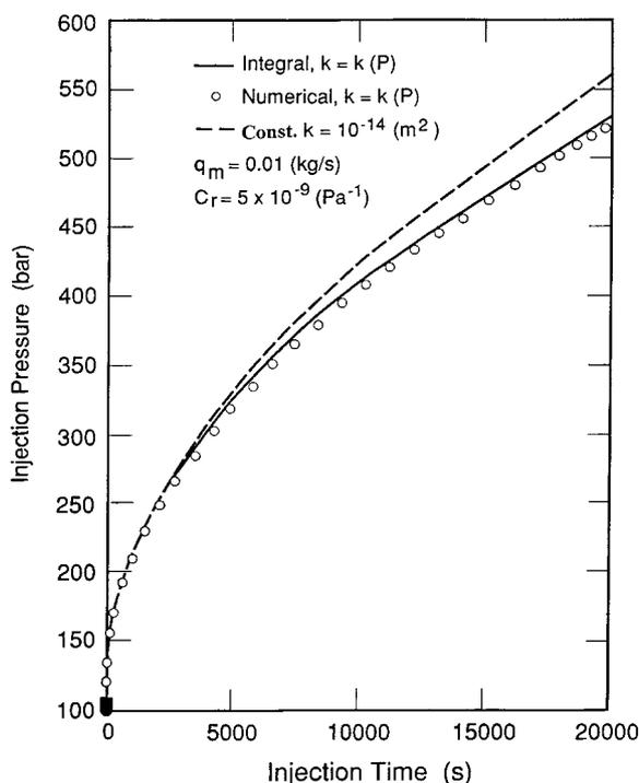
Fig. 4. Comparison of injection pressures calculated from integral, exact (constant permeability) and numerical solutions for linear flow in a permeability-dependent medium with permeability function (35).
