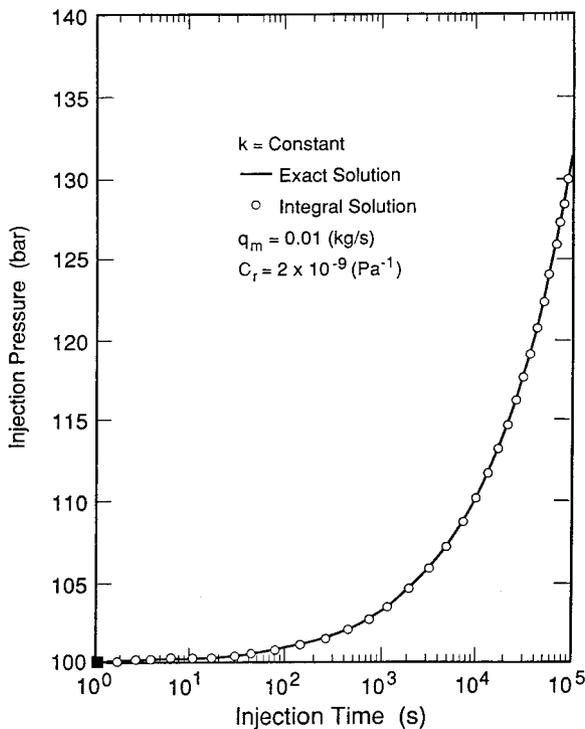
Fig. 2. Comparison of injection pressures calculated from integral and exact solutions for linear flow in a constant permeability medium.
