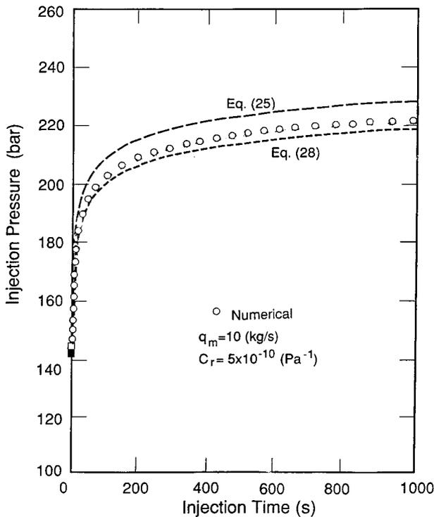
Fig. 6. Comparison of injection pressures calculated from integral and numerical solutions for radial flow in a weakly permeability-dependent medium with permeability function (34).
