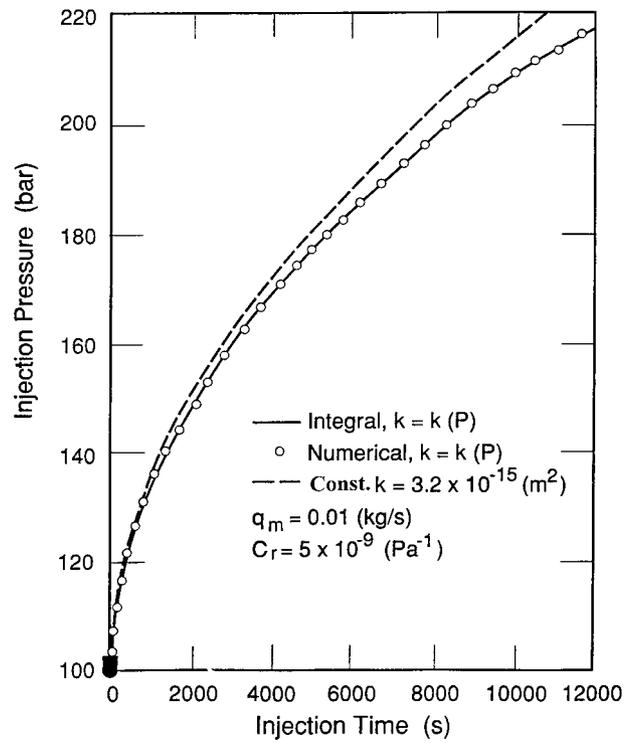
Fig. 3. Comparison of injection pressures calculated from integral, exact (constant permeability) and numerical solutions for linear flow in a permeability-dependent medium with permeability function (34).
