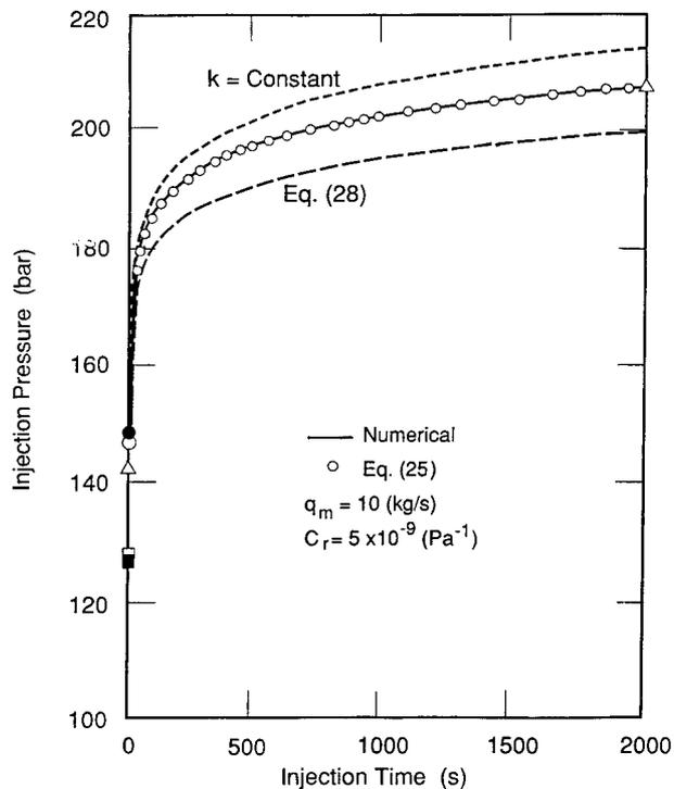
Fig. 5. Comparison of injection pressures calculated from integral and numerical solutions for radial flow in a strongly permeability-dependent medium with permeability function (34).
