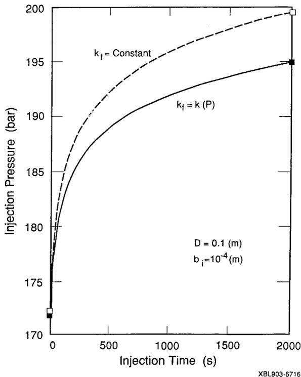
Fig. 9. Comparison of injection pressures in a radial fracture system with and without including effects of permeability changes.
