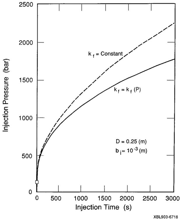
Fig. 8. Comparison of injection pressures in a linear fracture system with and without including effects of permeability changes.
