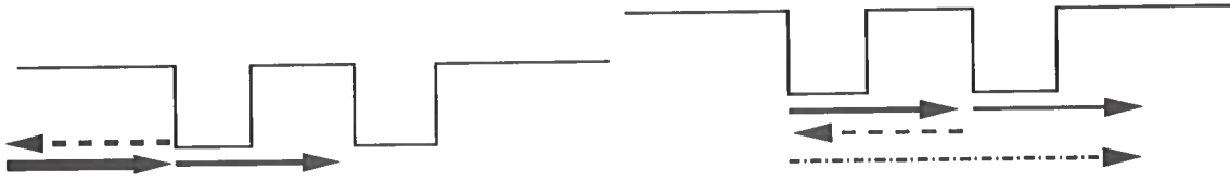
Figure 4.2. Side-view of paths for energy in grooved aluminum. Scattering of the incident surface wave causes loss of the transmitted field (left), but energy can be gained by being re-reflected in the direction of propagation (right).
