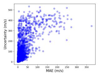
**Figure 5.** Correlation map between the absolute prediction error (MAE) and the corresponding uncertainty. The Pearson correlation is 0.727 (p-value is 1.0e-10), which shows a strong positive correlation between the absolute prediction error and the uncertainty.
