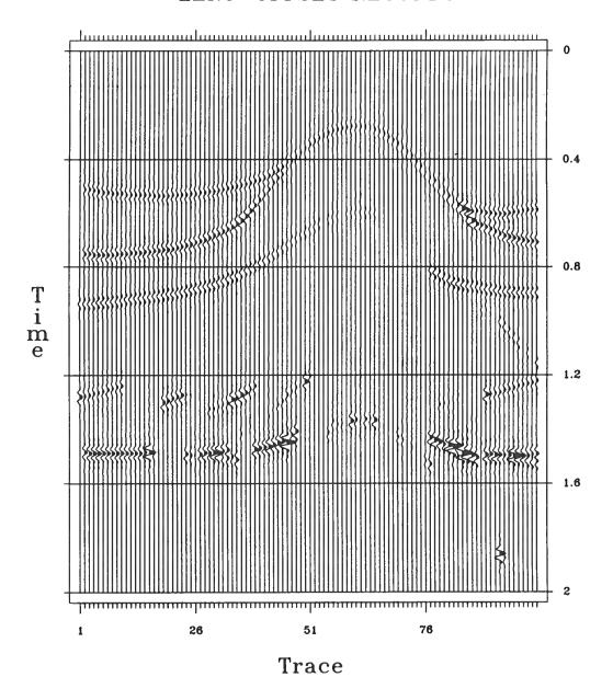
Figure 6: Pseudo zero-offset shot records for the 2.5-D model in Figure 3.
