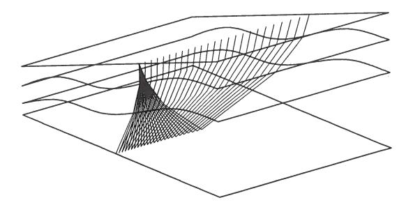
Figure 2: Perspective rayplot for a shot profile along strike.
