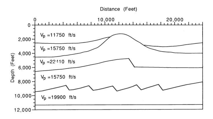
Figure 3: 2.5-D physical model (courtesy of Marathon Oil Company)
