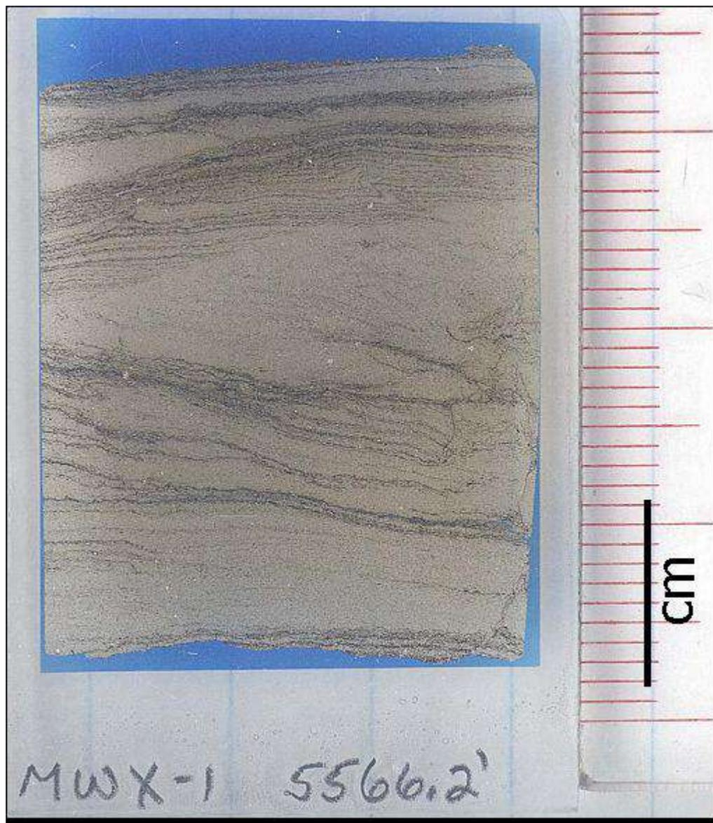
Figure 2-13 Thin section of a reservoir tight gas shaley sandstone sample (R-5566.2H). Depth 5566.2 ft, measured plug porosity is 3.7%, Klinkenberg corrected permeability is 0.009 mD and grain density  $2.71 \text{ g/cm}^3$ .
